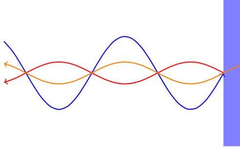
Figure 8.1: Reflection from a mirror can be minimized when the reflection from the front and back interfere destructively. This works for specific directions and wavelengths.
