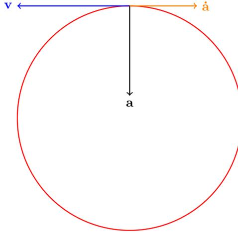
Figure 13.1: In a circular motion every derivative is a rotation by  $\pi/2$
