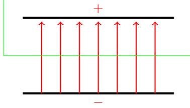
Figure 9.3: You need to apply an external force to hold the capacitor plates from collapsing on each other.
