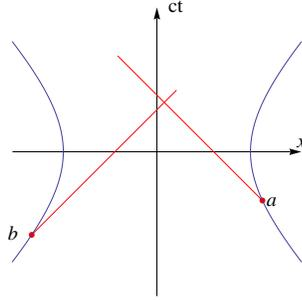
Figure 2.12: The world line of the two satellites are the blue lines. The intersection of the light cones is the event whose coordinates we seek. Since the orbits of the satellites are known, the events  $(a^0, a^1)$  and  $(b^0, b^1)$  are known given the proper times  $\tau_a$  and  $\tau_b$ .
