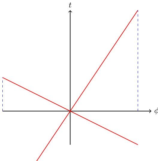
Figure 2.10: Minkowski space in rotating earth coordinates. It takes light different time, in the rotating frame, to complete a clockwise round-trip and counterclockwise round-trip.
