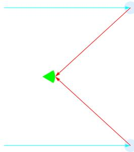
Figure 4.7: The cyan arrows represent light rays from the sun. The two small light-blue balls represent two water droplets. The red arrows are the reflected light rays in the direction of the rainbow caustics. The green eye represents the observer. Pilots sometimes see rainbows that are circular.
