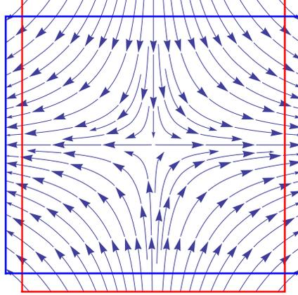
Figure 9.6: In the theory of elasticity a strain is described by a vector field. The figure shows the vector field associated with (uniform) contraction of  $y$  and dilation of  $x$ : Namely  $(x, -y)$ . The strain causes stress in the material. Energy is stored in it like in a compressed spring.
