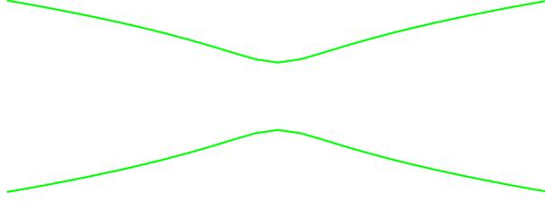
Figure 11.5: The waist of a Gaussian beam as function of  $z + ct$ .
