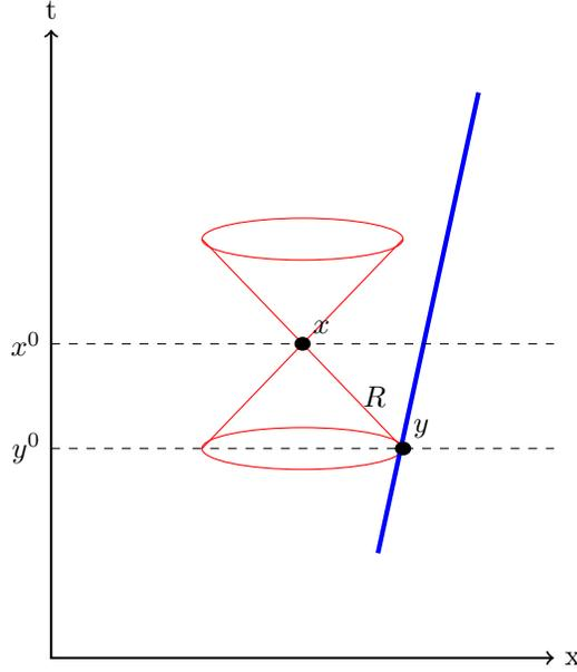
Figure 12.1: The blue line is the world line of the point source. The wave is observed at the black dot  $x$ . The backward light cone from  $x$  intersects the (blue) world line at the black dot  $y$ . Since the velocity is time like the point of intersection is unique.  $R$  is the 4 vector  $x - z(y^0)$ .
