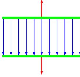
Figure 9.4: You need to apply a force to hold two oppositely charged capacitor plates apart (red arrows). If the arrow is in the  $z$ -direction,  $T^{zz} < 0$ . You get this sign if you think of the electric field lines as rubber band: As if the pressure is negative.
