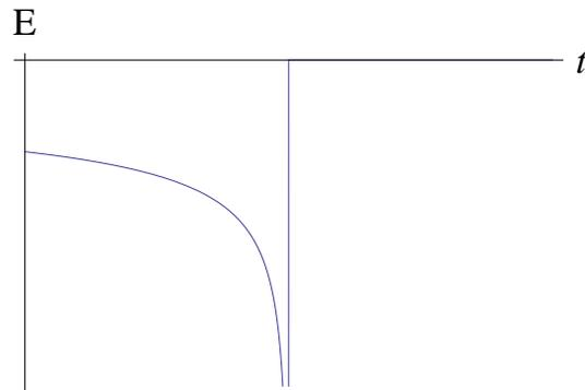
Figure 12.7: Blowup at finite time: The energy of a charged particle encircling the nucleus goes to  $-\infty$  in finite time.
