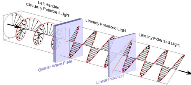
Figure 11.8: An arrangement that transmits right circular polarization.
