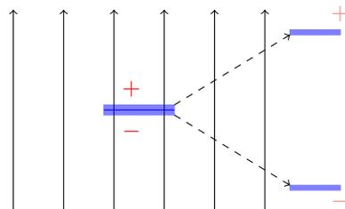
Figure 7.1: Put two thin metallic plates in contact in the field. The surface charge density on the plates is proportional to field strength. Separate the plates and measure the charge on the top plate. Define the field  $D$  as the maximal charge per unit area over all initial orientations of the plates.
