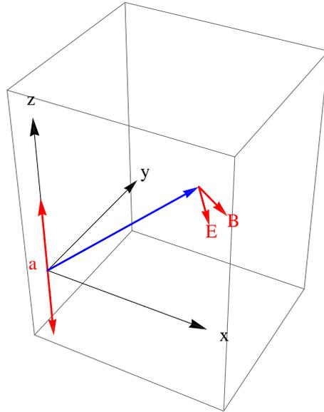
Figure 12.5: Dipole oriented along the z-axis and the associated fields.  $\phi$  is the angle between the z-axis and the blue arrow.
