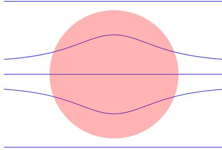
Figure 8.2: The figure illustrates a local coordinate transformation of the Euclidean plane, so that the image of straight lines become the curves in the figure. Such a coordinate transformation can be implemented by a choice of a suitable dielectric tensor  $\varepsilon$ . The corresponding dielectric, the reddish disk, is invisible.
