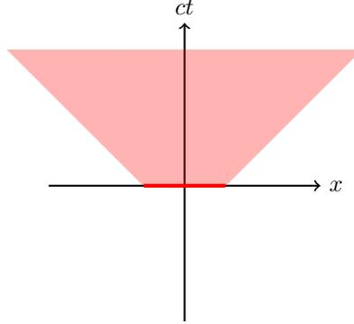
Figure 11.4: If the initial data,  $\phi_0$  and  $\dot{\phi}_0$  are localized in the red interval, the solution at later times lives in the forward light cone of the initial data. This is called the domain of influence of the initial (red) data. This statement holds in any inertial frame.
