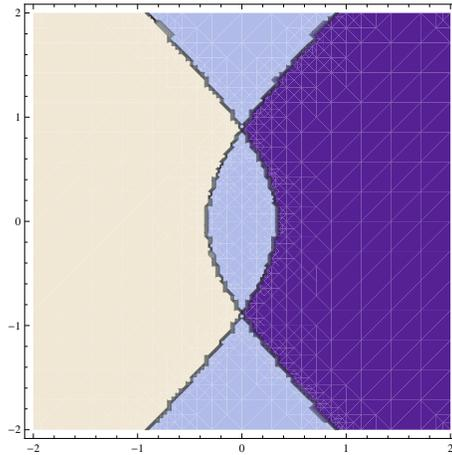
Figure 6.2: Maxwell's equation in 1+1 dimensions can be solved geometrically for arbitrary motion of the source. The figure illustrates the solution in space-time for two point sources undergoing constant acceleration. The field takes constant values in the different regions delineated by the orbits of the charges.
