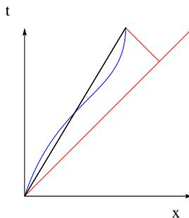
Figure 4.2: The world line is required to have time-like tangents—for the action to be real. The blue curve represents the variation of a world line with fixed end points. The black line maximizes the proper-time  $\tau$ . The red lines are light-like. The red path between the end points has zero proper-time.
