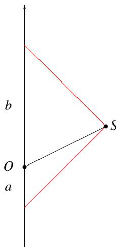
Figure 2.3: Wigner method of measuring space-like interval  $OS$  with a clock. The interval between the two space like events  $O$  and  $S$  is related to the clock readings  $a, b$ . The red lines in the figure are light-like.
