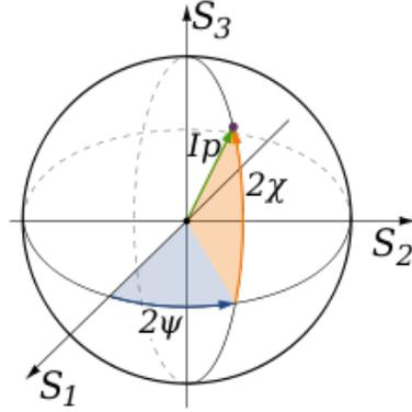
Figure 11.3: The Poincaré sphere associates with every point on the sphere a polarization. The north and south poles represent right and left circularly polarized light and the equator with linearly polarized light.
