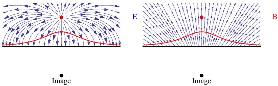
Figure 6.7: The red curve shows the surface charge density that allows the field to terminate at the surface. On the right one sees the response in the form of a magnetic field that seems to have a magnetic monopole at the image point. There is no real magnetic monopole anywhere, of course.
