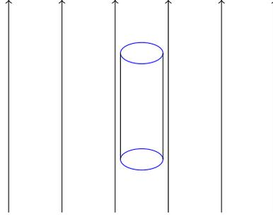
Figure 7.2: A thin superconducting cylinder expels the magnetic field by creating surface currents. Measuring the current gives  $H$ .
