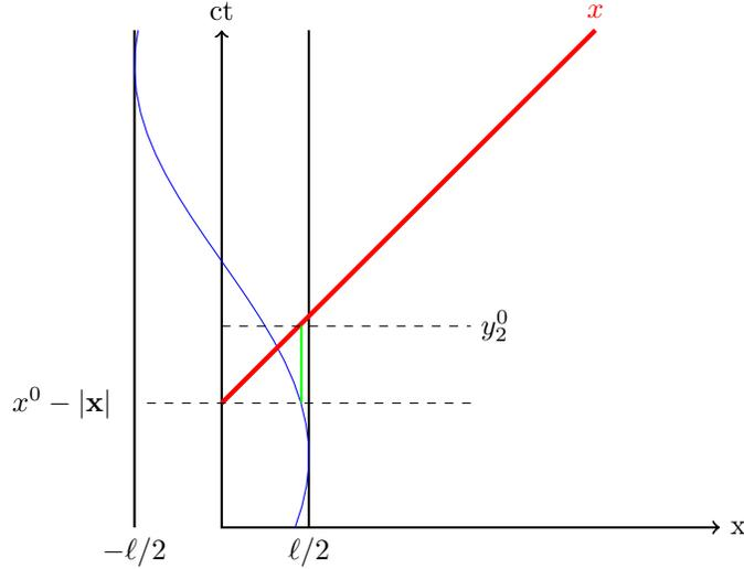
Figure 12.4: The blue line gives the orbit of the charge. The lowest order dipole approximation is  $x^0 - |\mathbf{x}|$ . A better approximation is  $y_2^0$  which takes into account the position of the charge at  $x^0 - |\mathbf{x}|$ . One could get better approximations by also taking into account the velocity of the charge.
