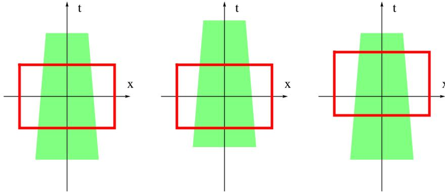
Figure 9.7: The action remains the same when the fields and the integration box are both shifted in space-time. For a small shift the change in action can be split into two virtual shifts: A shift of the field with the box held fixed, shown in the middle figure, and a shift of the box with the field held fixed field, shown on the right.
