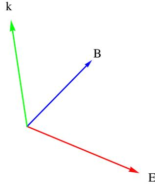
Figure 11.1: The triad of  $\mathbf{E}$ ,  $\mathbf{B}$ ,  $\mathbf{k}$  for a plane wave. The wave propagates in the  $\hat{\mathbf{k}} = \hat{\mathbf{E}} \times \hat{\mathbf{B}}$  direction
