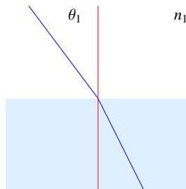
Figure 4.5: The change in direction of a ray when  $n$  jumps is determined by Snell's law
