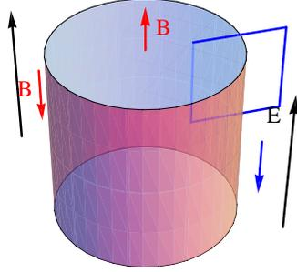
Figure 6.5: A cylinder of a (non-trivial) topological insulator is immersed in vacuum (trivial insulator). A uniform electric field  $\mathbf{E}$  in the axial direction leads to response in a magnetic field inside the cylinder
