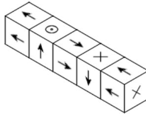
Figure 9.9: Halbach array gives a large magnetic field above the array and small one below it.
