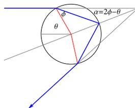
Figure 4.6: The blue line shows a ray undergoing one internal reflection in a drop of water. The impact angle  $\theta$  is defined in the figure. The outgoing ray is focused near the maximum  $2\phi - \theta$ . This partial focusing is called a caustic. This gives the direction of the rainbow.
