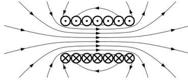
Figure 9.5: The magnetic field lines of a solenoid run parallel to the solenoid axis. As a consequence the stress in the radial direction  $T^{\rho\rho} > 0$  inside the solenoid. You get the right sign if you replaced the field lines by rubber bands: Stretched rubber bands along the  $z$ -axis, that fan out in the radial direction, will lead to a positive pressure in the radial direction and negative pressure in the axial direction.
