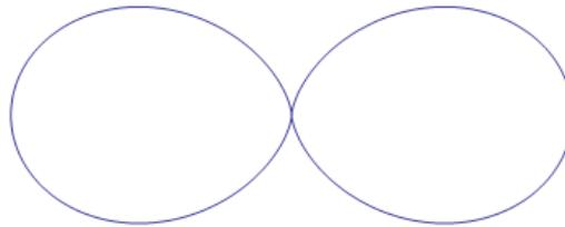
Figure 12.6: Polar plot of the power radiated by a dipole antenna as function of the angle, Eq. 12.51. The maximal power is radiated in the plane perpendicular to the dipole.
